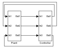
Your starting point in developing a combined plant and controller system model is to model the combined system as two subsystems in closed-loop simulation. As your design progresses, you can use Simulink external mode with standard Real-Time Workshop targets (such as GRT or ERT) to help you model the controller system separately from the plant.
