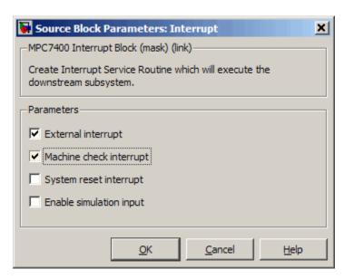
To test your interrupt configuration in simulation, select **Enable simulation input** on the block dialog box and then input a signal to the block to simulate the external interrupt.
