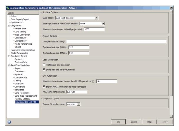
When you designate a block function as inline, the compiler replaces each call to a block function with the equivalent function code from the static run-time
