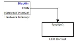
In this model, the Hardware Interrupt block installs a task that runs when it detects an external interrupt. This task performs the specified function with an LED.
