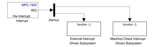
Here is the block mask showing the external and Machine check interrupts selected.
