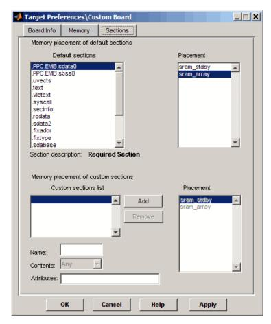
Within this pane, you allocate the memory needed for the **Default sections** and **Custom sections**.
