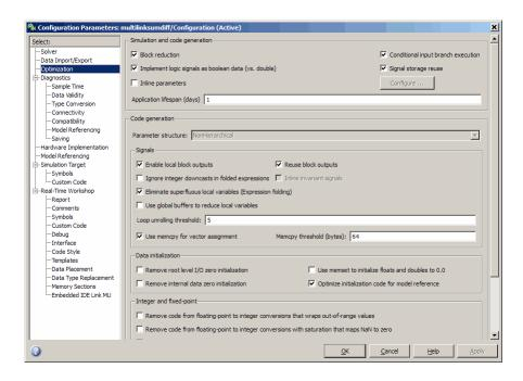
These options are typically selected for Real-Time Workshop software to provide optimized code generation for common code operations:
