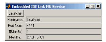
Information in the window provides details about the service. Clicking **Launcher** opens the MULTI Launcher utility.
