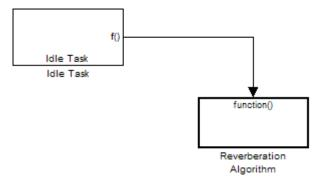
The function generated for this task normally runs in free-running mode—repetitively and indefinitely. Subsystem execution of the reverberation function is the same as the subsystem described for the Free-Running DSP/BIOS Task. It is data driven via a background DMA interrupt-controlled ISR, shown in the following figure.
