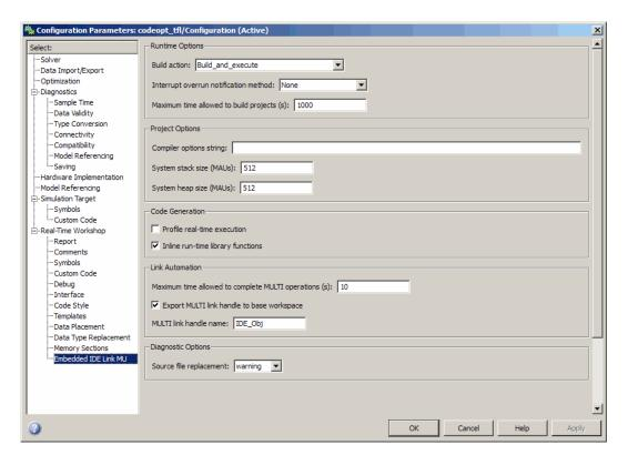
In the **Select** tree, the categories provide access to the options you use to control how Real-Time Workshop software builds and runs your model. The first categories in the tree under Real-Time Workshop apply to all Real-Time Workshop targets and always appear on the list.
