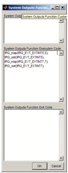
Generating code from your model that includes the System Outputs block adds the enabling and mapping code to your project so the interrupts work. The following figure shows a top-level model c6000\_hwi\_interrupts that includes the System Outputs block in the Function-Call Subsystem2 submodel.
